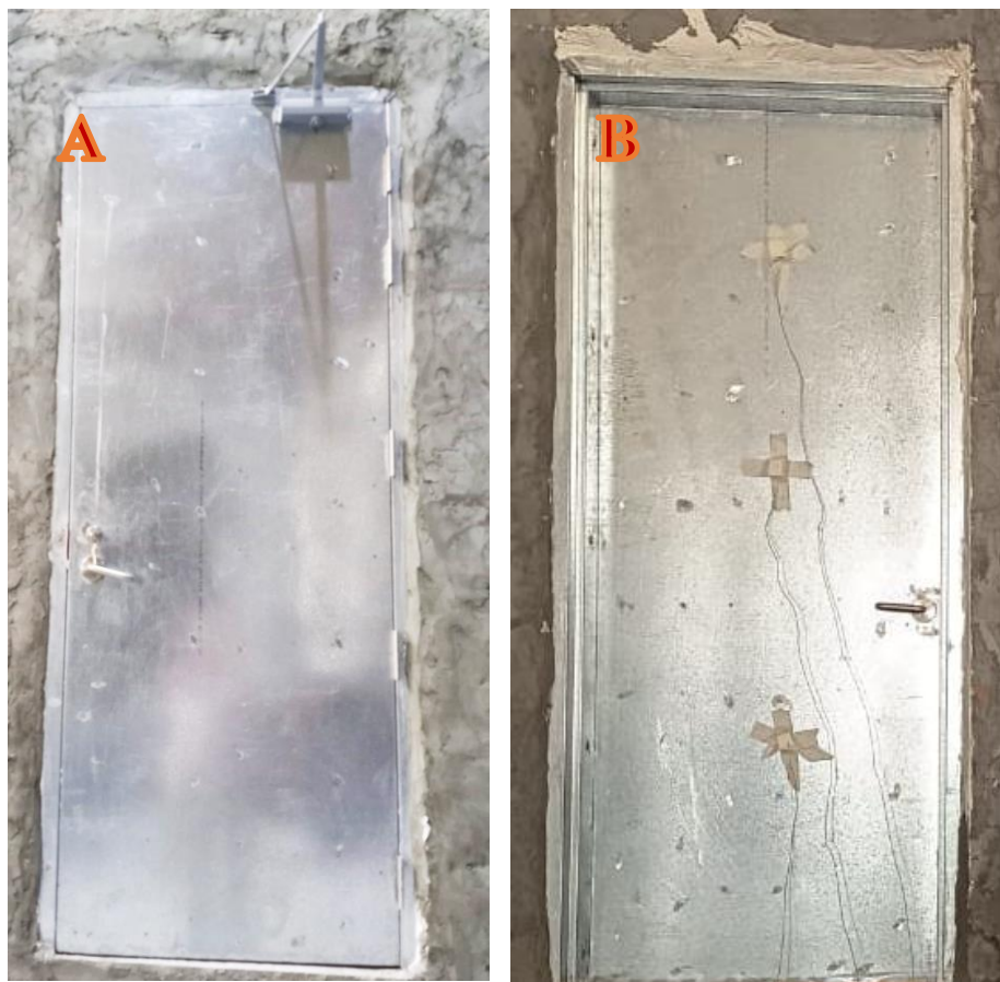
Figure 1: Photos of the door assembly, (A) Exposed face, (B) Unexposed face
