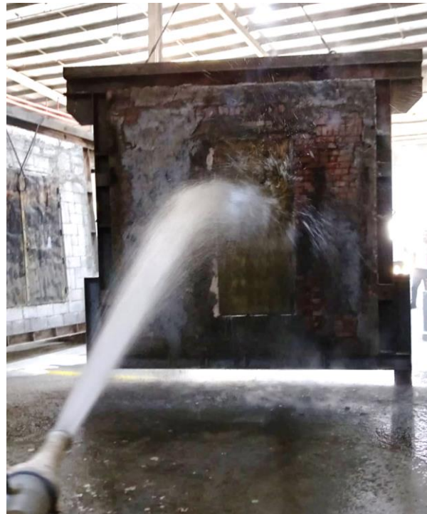
Figure 8: Hose stream test after 90 minutes of fire endurance
