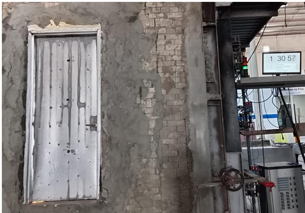
Figure 6: The end of the fire endurance test after 90 minutes.
